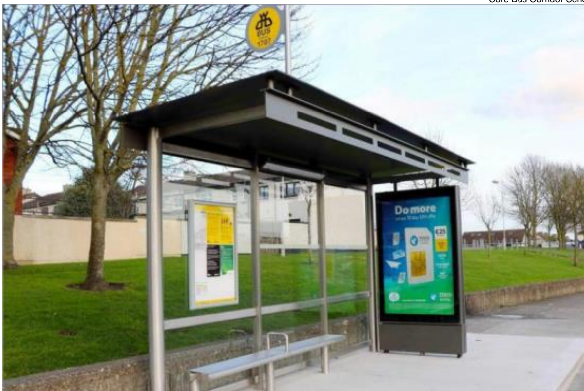
Figure 2.10 Standard 3 Bay Reliance Mark Shelter with full width advertising panel
