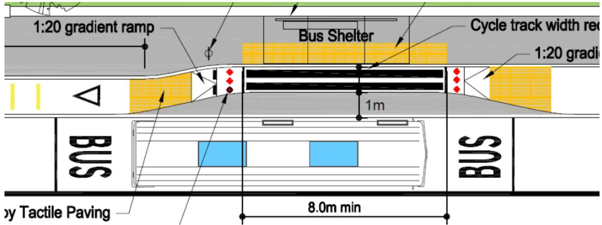
Figure 4.15: Alternative Shelter Location Back of Footpath (Narrow Island with Adequate Footpath Widths)
