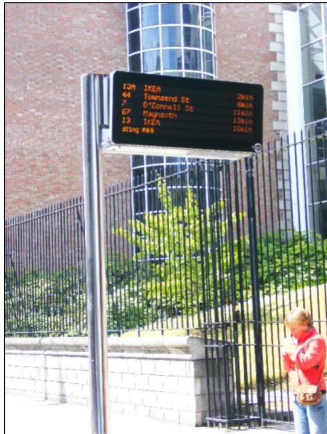
Figure 12.1: Illustration of RTPI Display at Bus Stop
