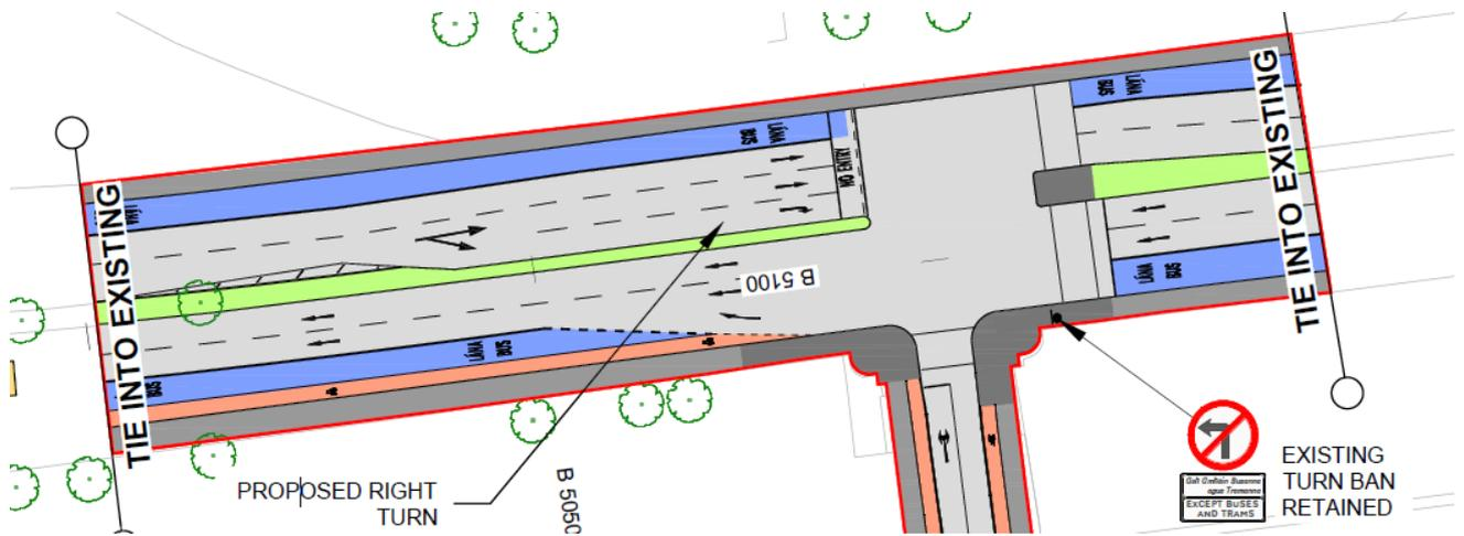
**Figure 3.8: The Preliminary Design of the Proposed Scheme at the Chapelizod Bypass which Ties in with the Existing Layout**
