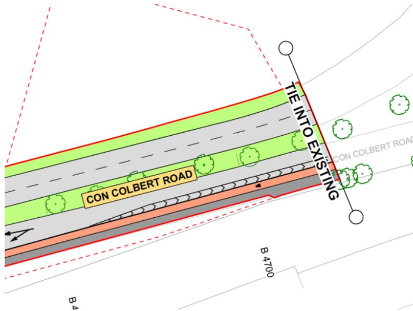
Figure 3.6: Preliminary Design of the Proposed Scheme Tie-In with the Lucan to City Centre Core Bus Corridor Scheme
