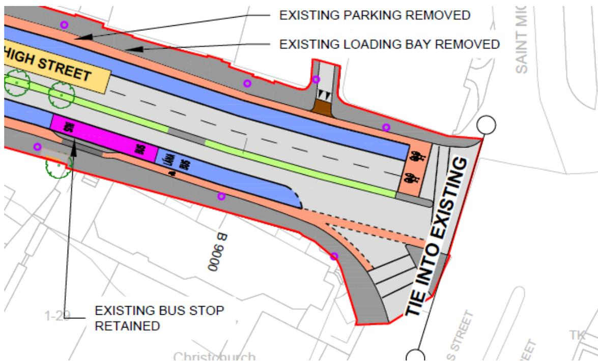
**Figure 3.12: The Preliminary Design of the Proposed Scheme at the Junction of High Street and Winetavern Street with the Existing Layout**
