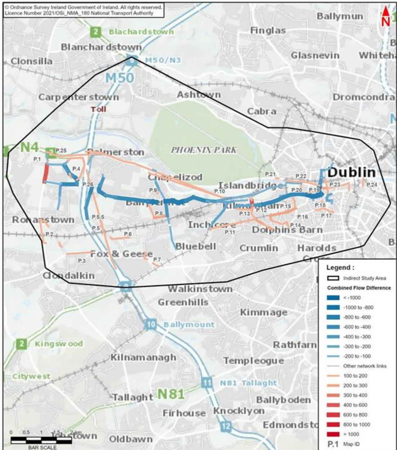
Figure 5.8: Flow Difference on Road Links (DM versus DS), PM Peak Hour, 2028 Opening Year
