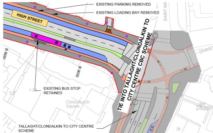
**Figure 3.13: Indicative Coordinated Design of the Expected Overall Arrangement in a Scenario in which Both Schemes Have Been Implemented**
