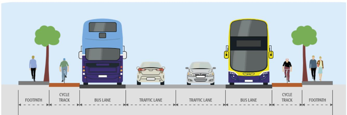
**Figure 4.1: Typical CBC Cross Section**
