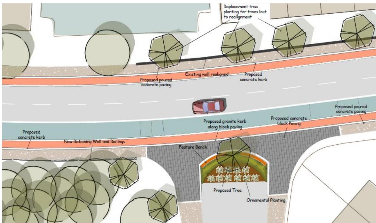
Figure 14.14: Road Closure at End of O'Hogan Road with Local Enhancement
