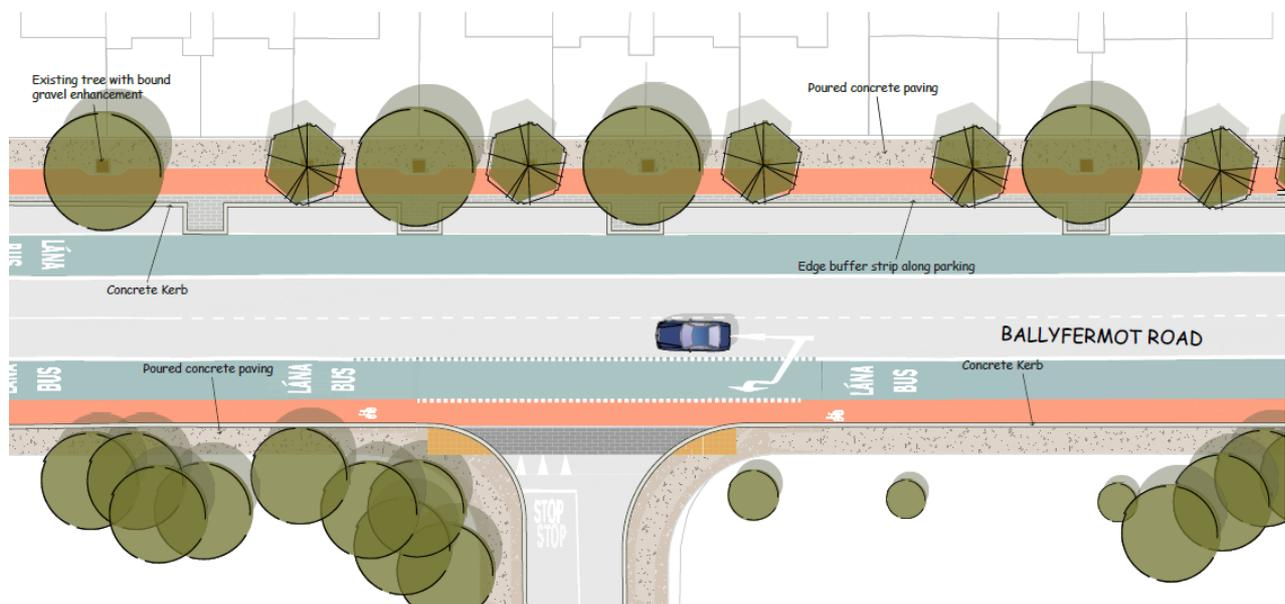
Figure 14.6: Rearranged Parking and Cycle track to Front of Residential Properties East of Cloiginn Park
