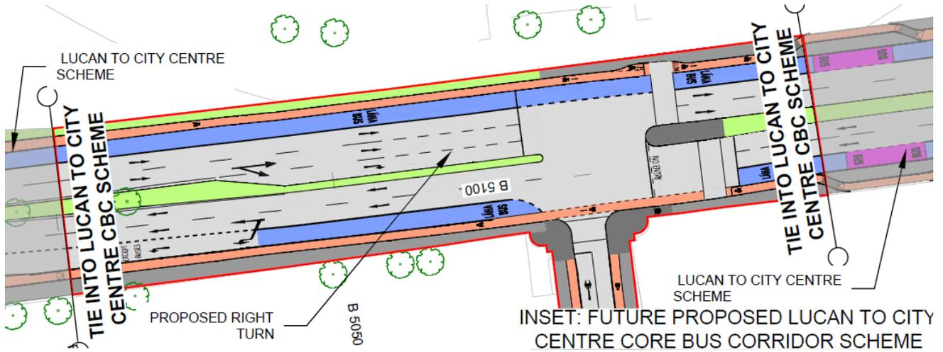
**Figure 3.9: Indicative Coordinated Design of the Expected Overall Arrangement in a Scenario in which Both Schemes have Been Implemented**
