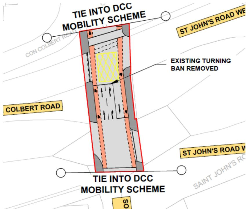
Figure 3.10: The Preliminary Design of the Proposed Scheme at Island Bridge which Ties in with the Existing Layout
