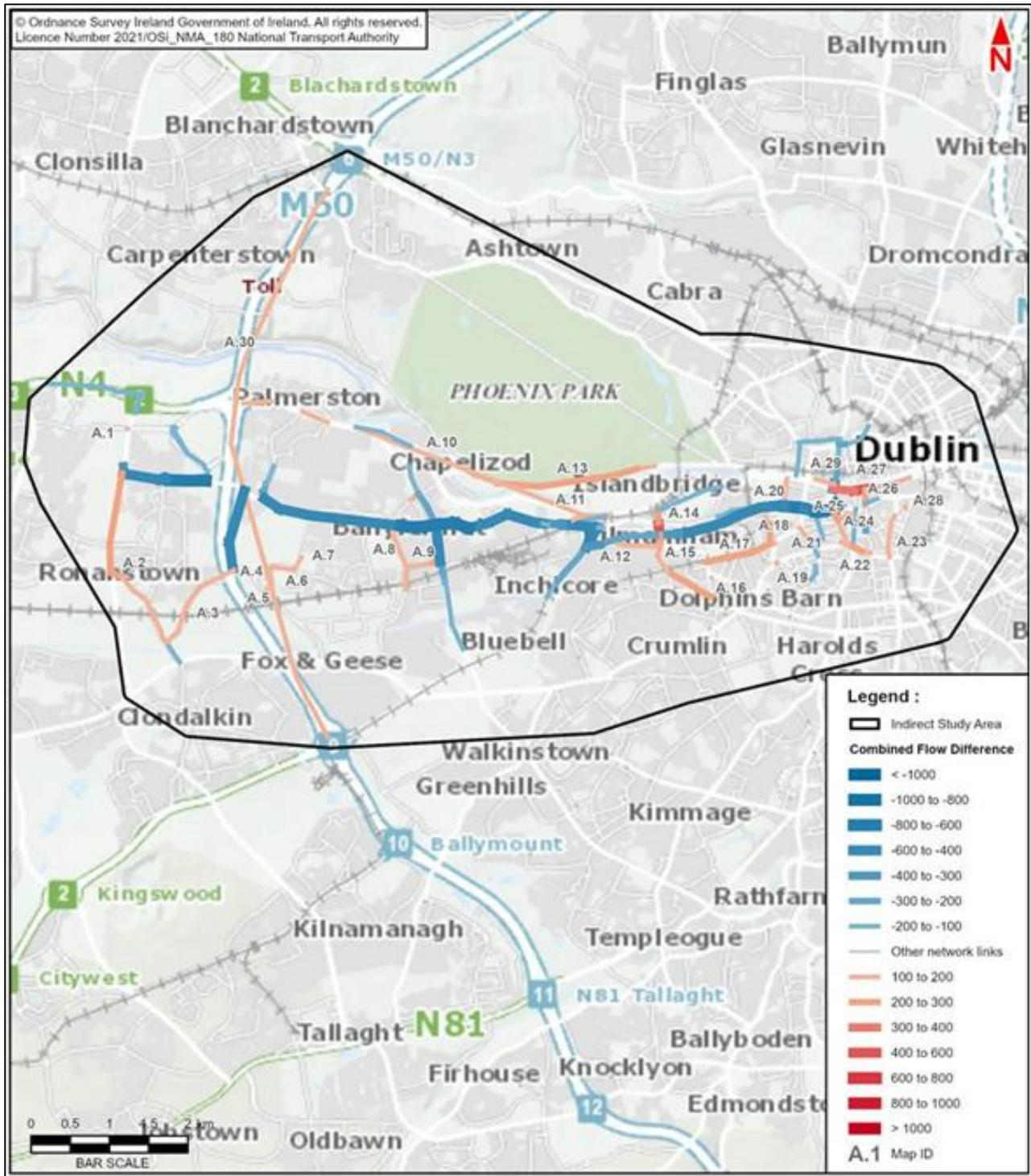
Figure 5.7: Flow Difference on Road Links (DM versus DS), AM Peak Hour, 2028 Opening Year
