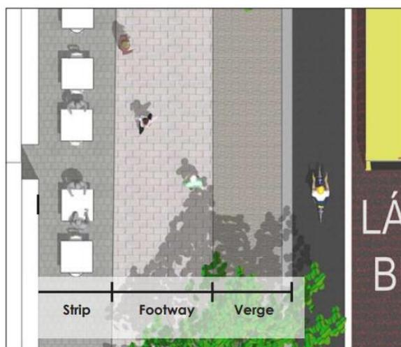
Figure 4.4: Key Components of the Footpath
