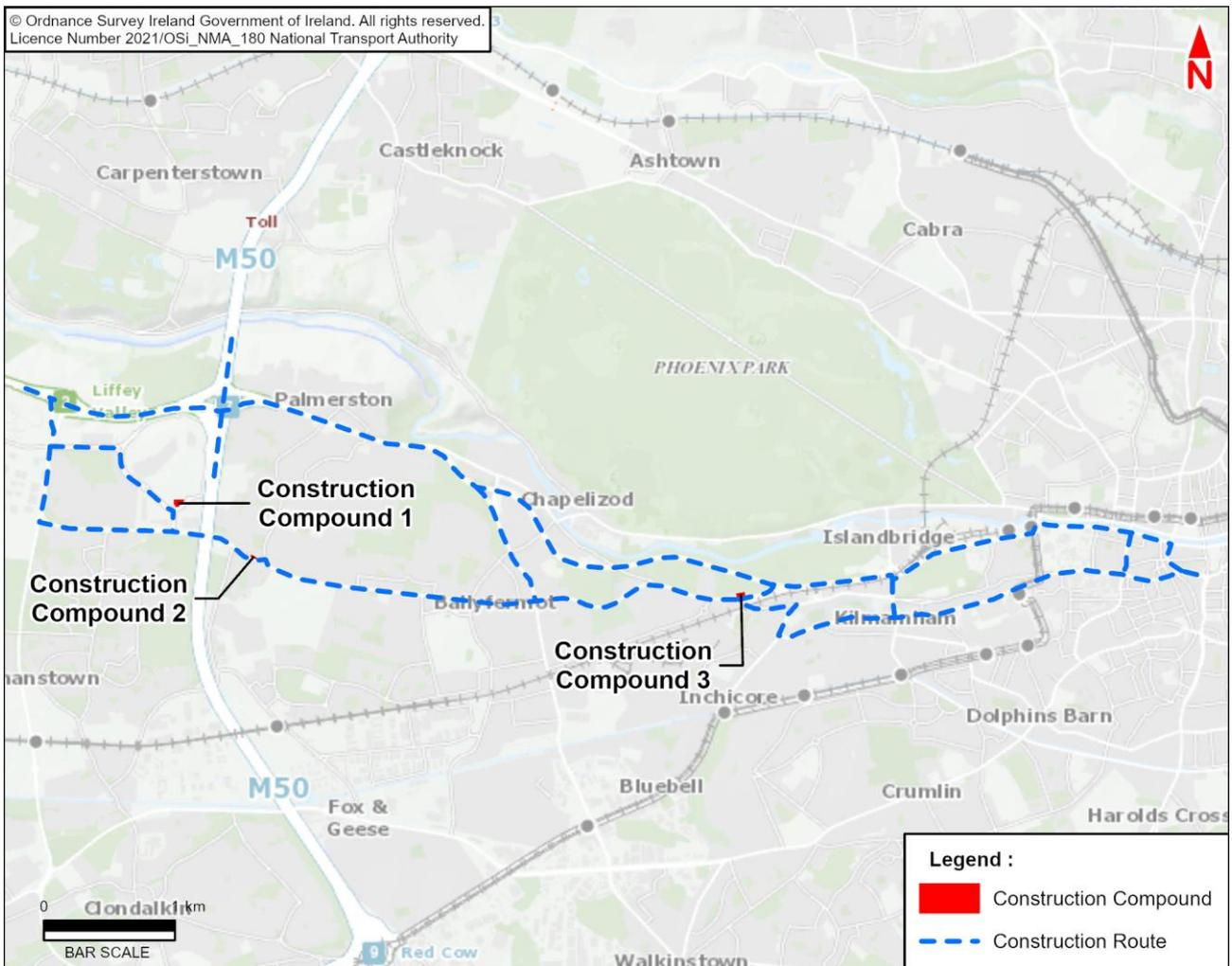
Diagram 6.3: Proposed Construction Routes and Main Compound Locations
