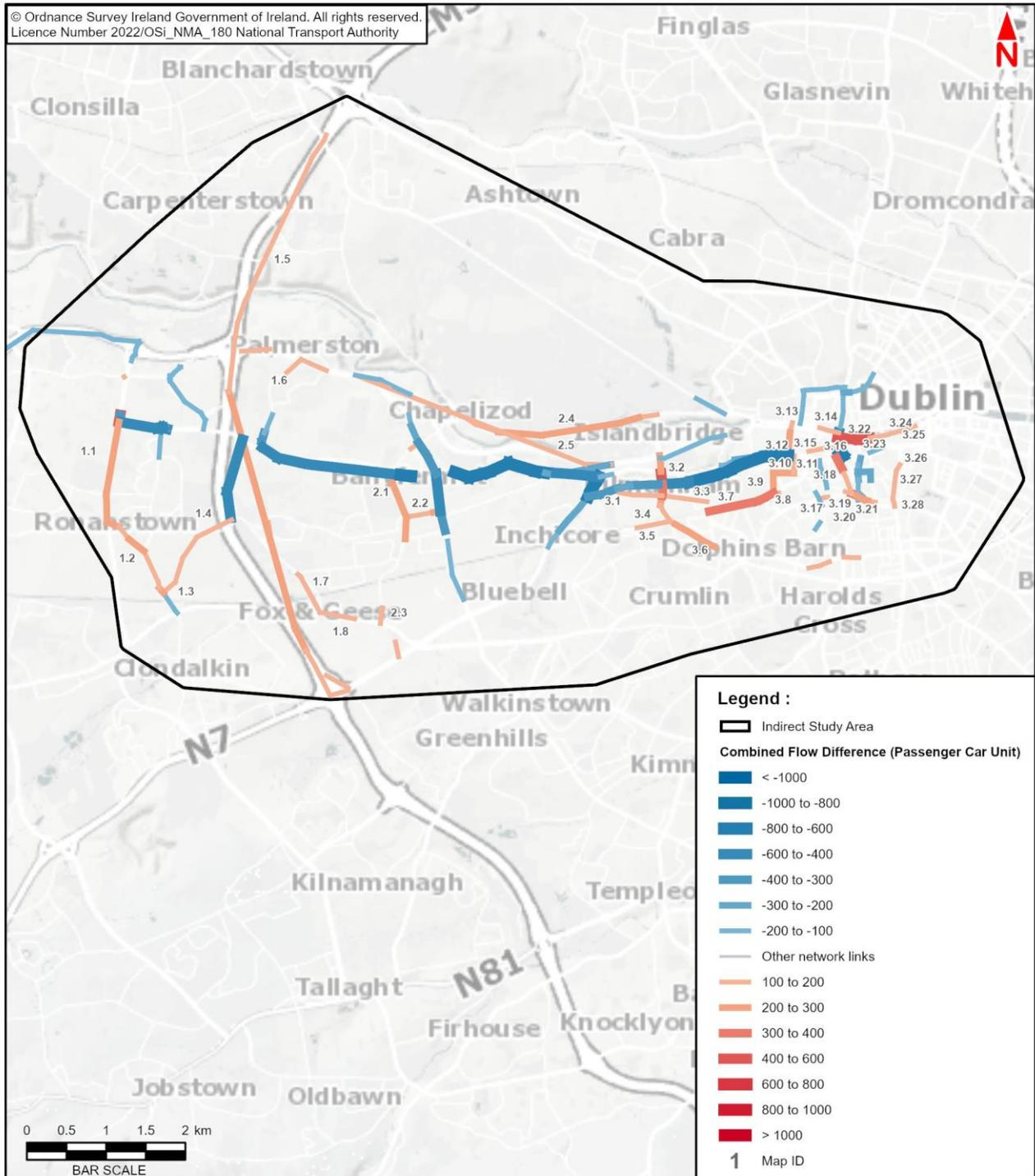
**Diagram 6.24: Flow Difference on Road Links (Do Minimum vs Do Something), 2028 Opening Year - AM Peak Hour**
