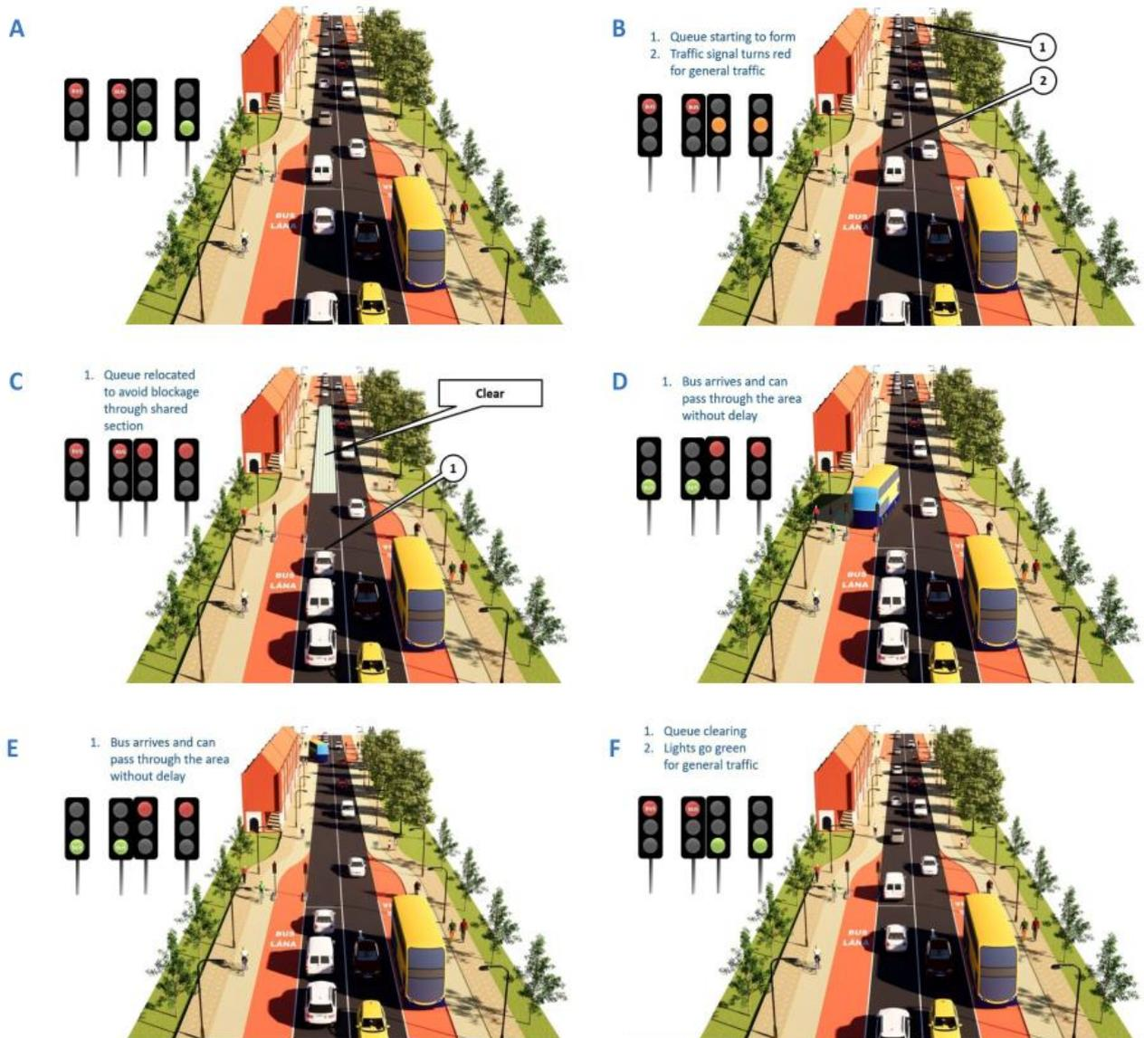
Image 4.17: Signal Controlled Priority Schematic Operation (Source: PDGB)
