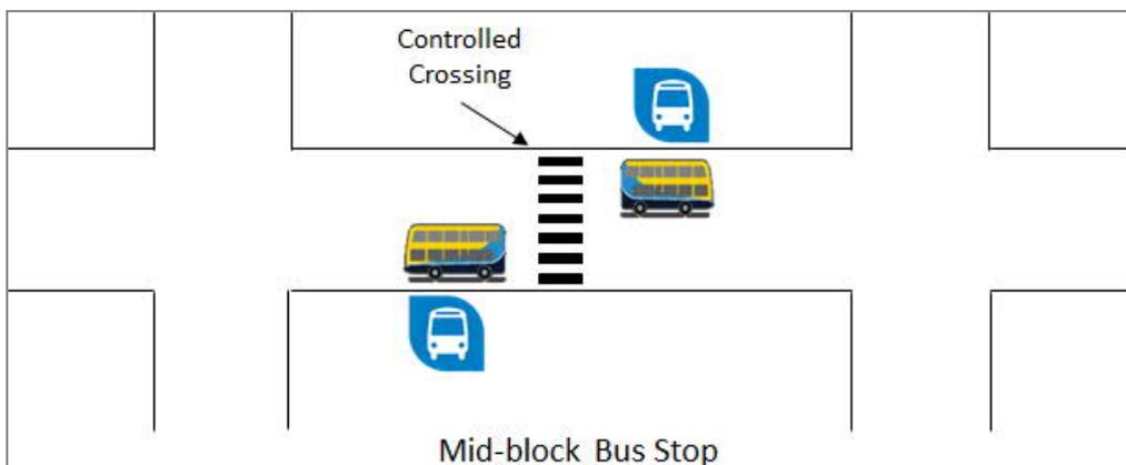
**Figure 5.10** Mid-block bus stop optimum layout.
