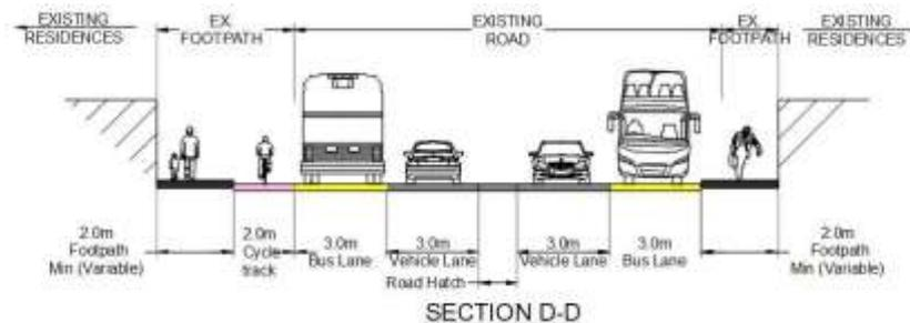
**Figure 7.20: CCT04 Cross-Section D-D**
