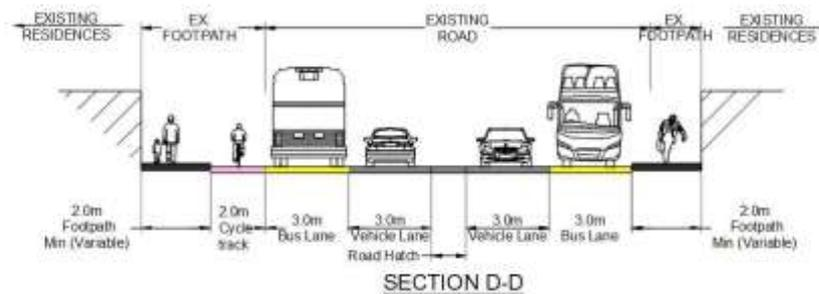
**Figure 7.44: CCT09 Cross-Section D-D**
