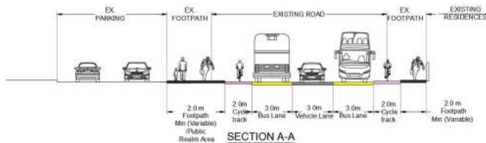
**Figure 6.15: BF04 Cross-Section A-A**
