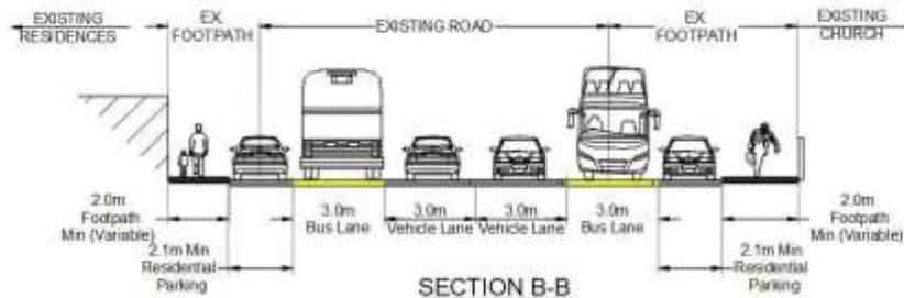
**Figure 7.13: CCT03 Cross-Section B-B**
