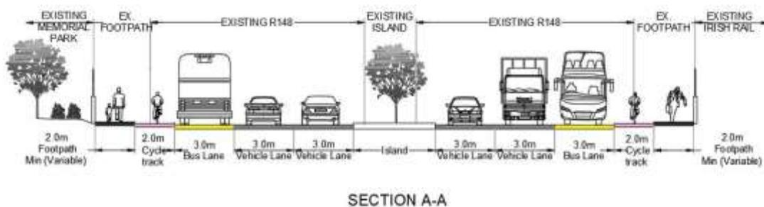
**Figure 7.17: CCT04 Cross-Section A-A**
