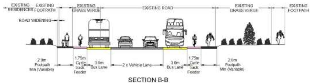
**Figure 5.6: LV01 Cross-Section B-B**
