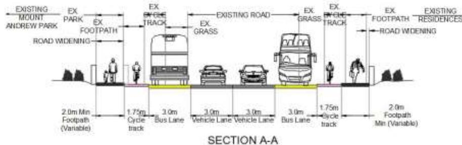
**Figure 5.10: Section 1 Full Route Option Cross-Section A-A**
