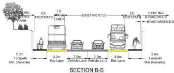
**Figure 7.5: CCT01 Cross-Section B-B**
