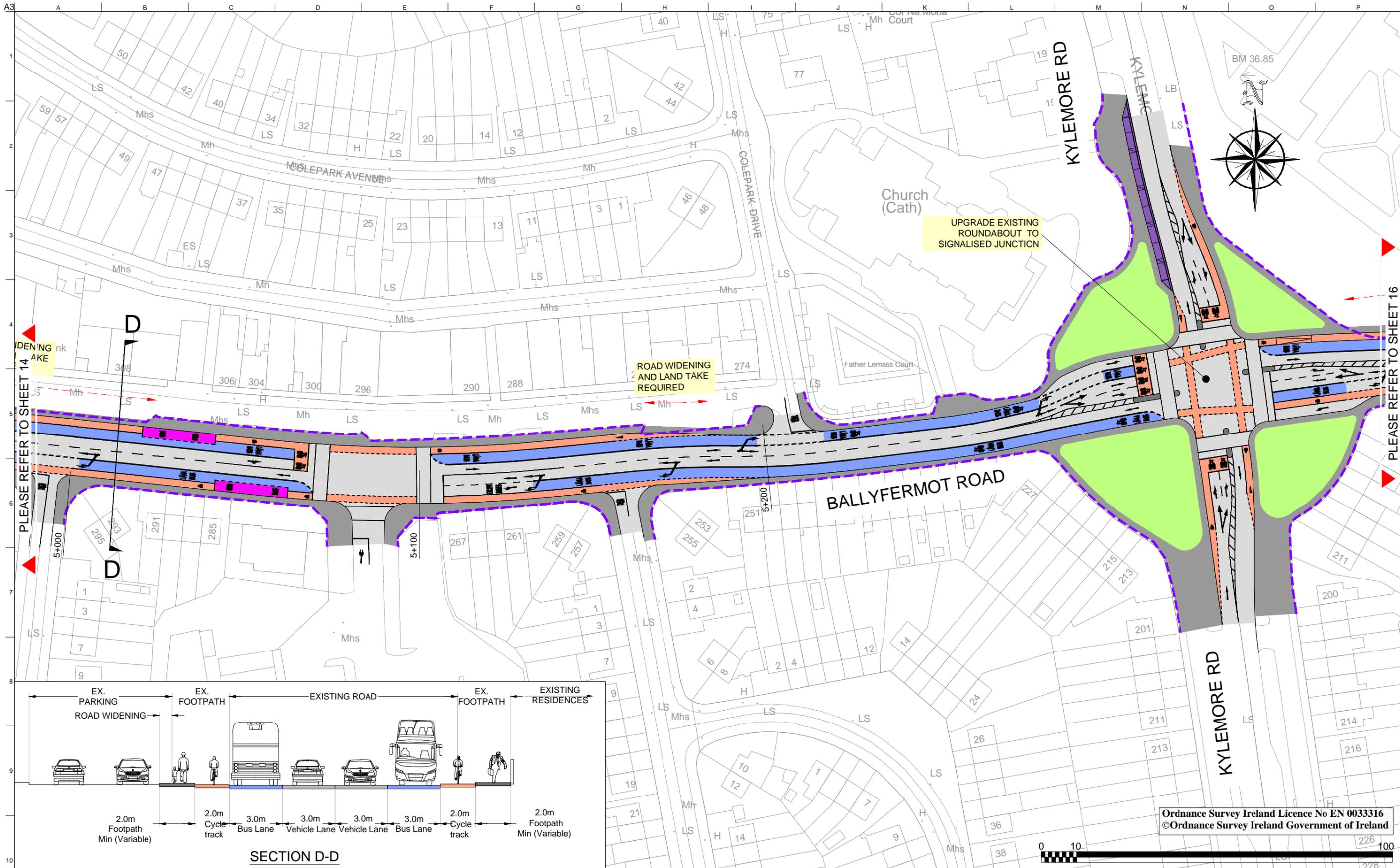
UPGRADE EXISTING ROUNDABOUT TO SIGNALISED JUNCTION
