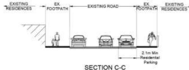
**Figure 7.14: CCT03 Cross-Section C-C**
