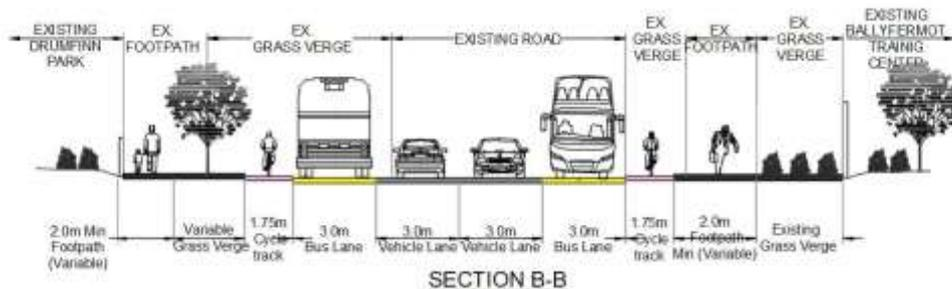
**Figure 6.5: BF01 Cross-Section B-B**
